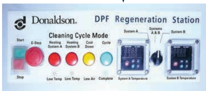
The simple, automated control panel of the DPF Regeneration Station.
