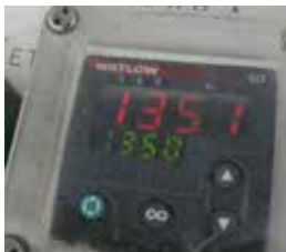
Green# = Set Point Red# = Heater Temp
