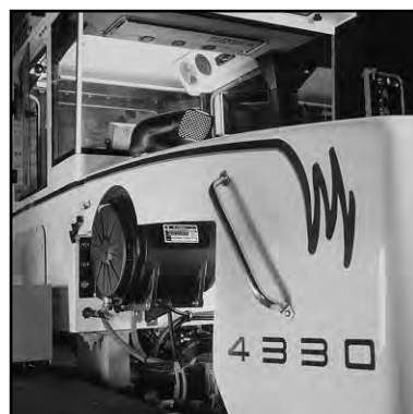
The EPG Air Cleaner, which fits neatly under the hood of this Tyler Ag Sprayer, protects the engine with its powerful air filtration capability. The Radial Seal Sealing Technology means a reliable seal even in rugged environments and fast filter change-out. (Above: the hood of the vehicle is up. Left: the hood is down.)
