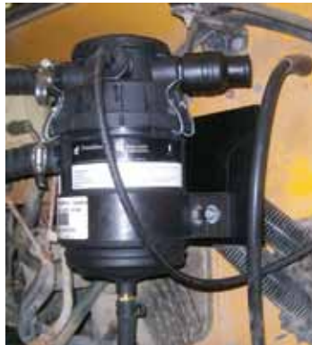
FIGURE 4 SPIRACLE SYSTEM ON A SCHOOL BUS
