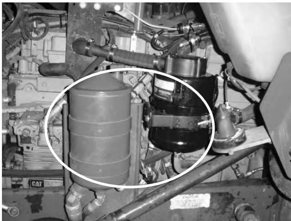
Example 5: Fabricated mount to existing power steering reservoir bracket
