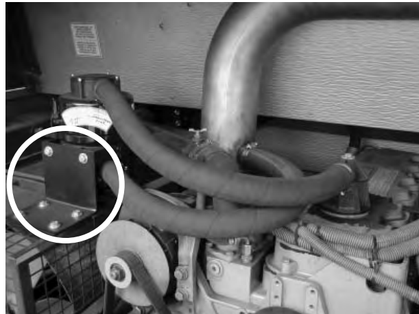
Example 2: Fabricated new mounting bracket
