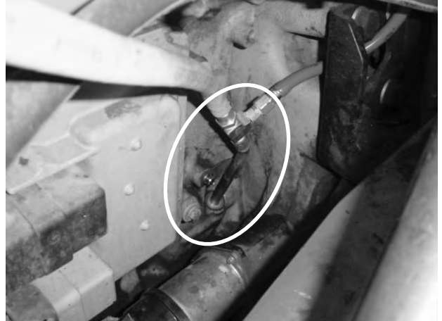
Example 4: Unused dipstick drain hole used for Spiracle oil drainback.
