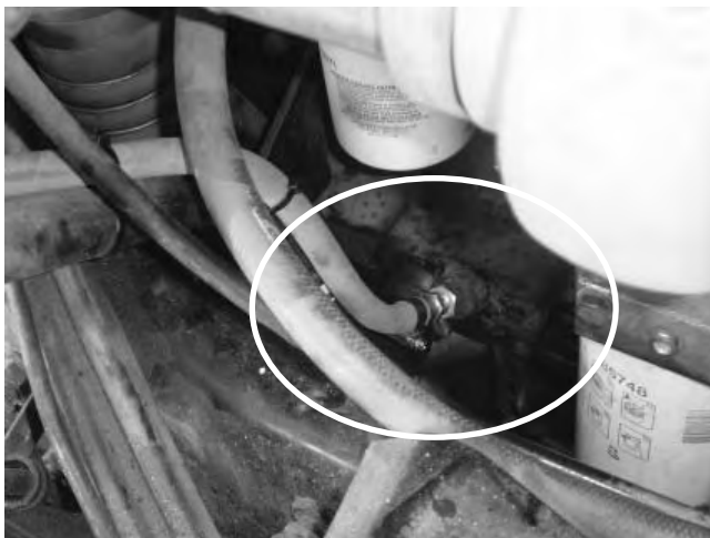
Example 3: Check valve installed in existing engine block port.
