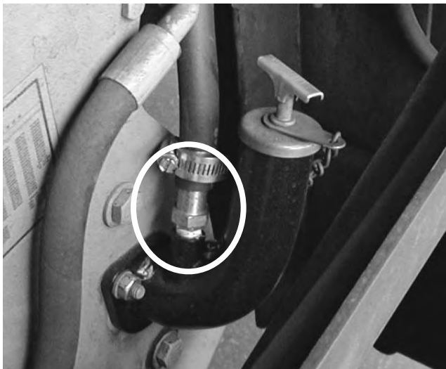
Example 3: Check valve installed in existing engine block port.
