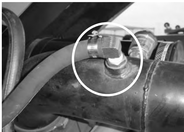
Example 1: Existing NPT adapter on clean air duct.
