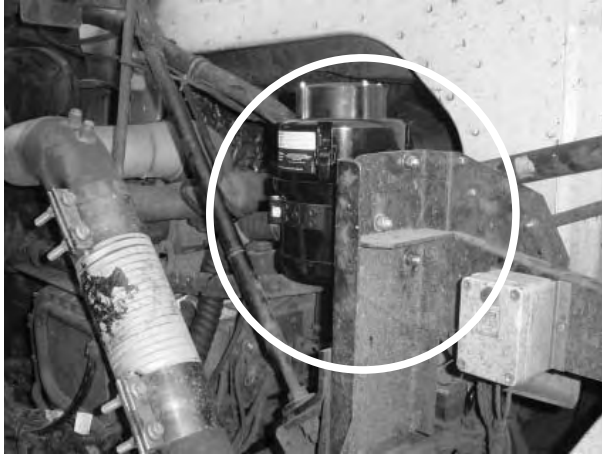
Example 5: Fabricated mount to existing power steering reservoir bracket
