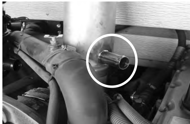
Example 2: Tubing with beaded end welded onto intake pipe
