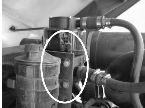
Example 2: Fabricated new mounting bracket
