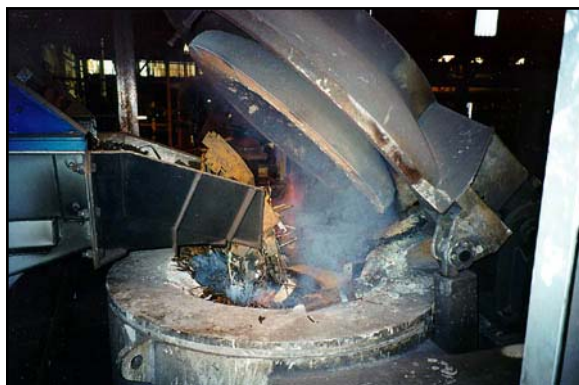
In this furnace application, Donaldson Dura-Life filter bags yielded twice the life -- 3000 hours of operation vs. 1500 -- compared to standard poly bags.
