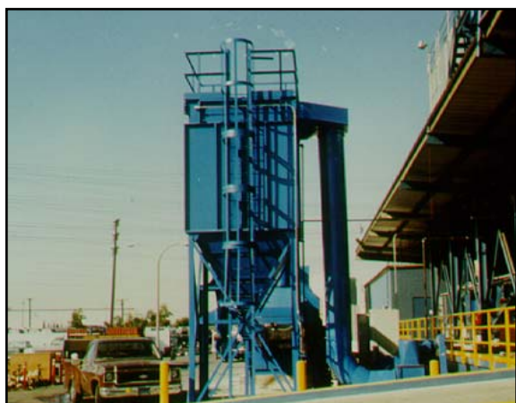
Dura-Life filter bags in a Donaldson Torit HPT dust collector are yielding 5X longer life than conventional polyester and passing the ongoing stack emissions tests.
