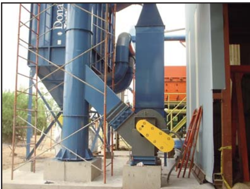
Dura-Life filter bags in this Donaldson Torit Modular Baghouse don't plug at this automotive parts maker.
