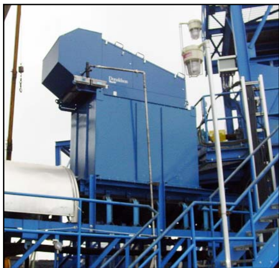
The Dalamatic Insertable is a dust collector designed to fit into existing ducts and silos to collect dust at the point of generation.
