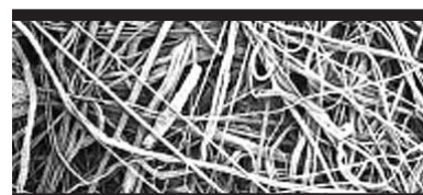
SEM of Ultrapolyplea PP100 depth filter element
