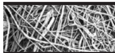
SEM of Ultrapolyplea® depth filter
