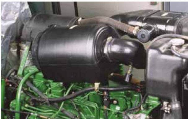
This EPG RadialSeal™ Air Cleaner is part of a complete Donaldson intake system. The entire engine air intake system is made of molded plastic. Between the intake scoop and the air cleaner are Donaldson Strata™ tubes, which provide pre-cleaning. Particulate from this stage is scavenged off and out through the exhaust system. In this system, the EPG air cleaner provides the second stage of cleaning.
