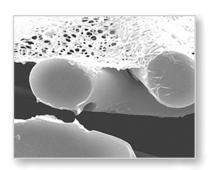
Ultra-Web nanofiber media has submicron diameters and small interfiber spaces, resulting in the contaminant being captured on the surface of the media, greatly improving filtration efficiency and making effective pulse cleaning possible
