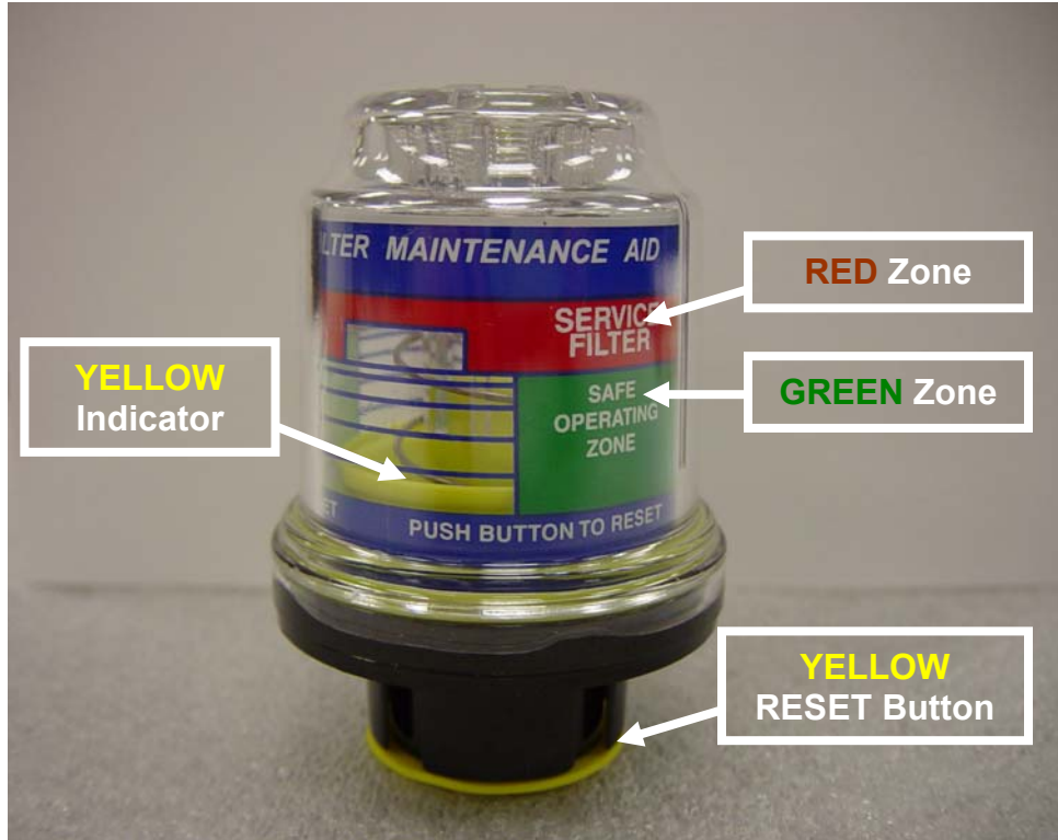
Figure 4-1. FILTER MAINTENANCE AID – (ABOVE) “YELLOW Indicator” position relative to SAFE OPERATING ZONE (“GREEN Zone”) or SERVICE FILTER (“RED Zone”) markings defines current filter condition and pushing “YELLOW RESET Button” resets indicator. (BELOW) FMA unit is mounted to inner frame of IBF assembly and can be viewed through access window in the upper fairing.
