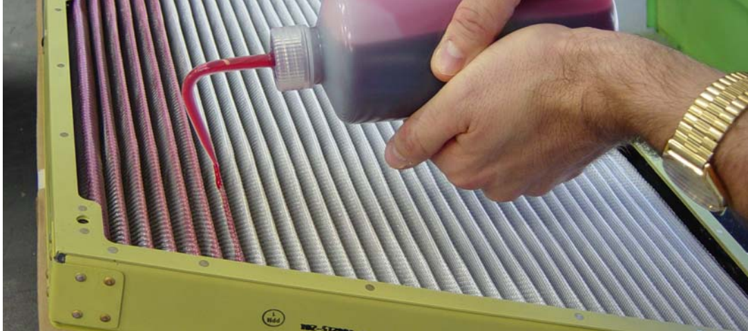
Picture 4: Oiling Filter Media
