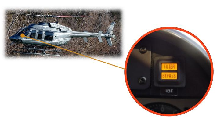
Pilot commands the bypass door to open to increase engine airflow until clear of debris conditions.
