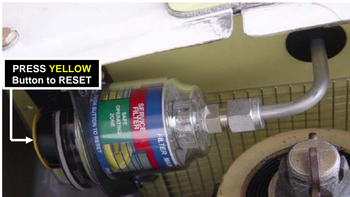
Picture 8-6: FMA / RESET LOCATION - unit is mounted to bottom of IBF floor assembly and is accessed through RH access door on air induction cowling.
