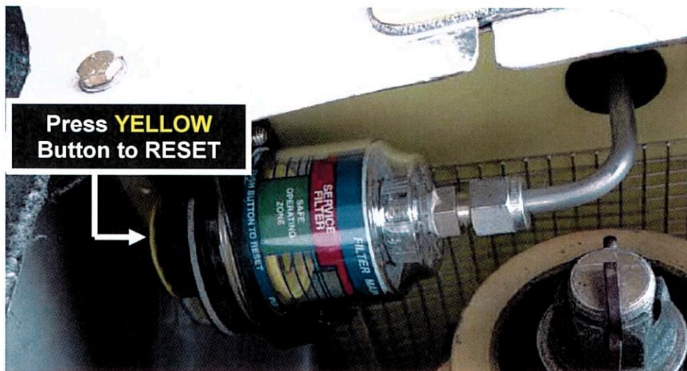
Figure 2-1. FILTER MAINTENANCE AID – (ABOVE) “YELLOW Indicator” position relative to SAFE OPERATING ZONE (“GREEN Zone”) or SERVICE FILTER (“RED Zone”) markings defines current filter condition and pushing “YELLOW RESET Button” resets indicator. (BELOW) FMA unit is mounted to bottom of IBF floor assembly and is accessed through RH access door on air inlet cowl assembly.
