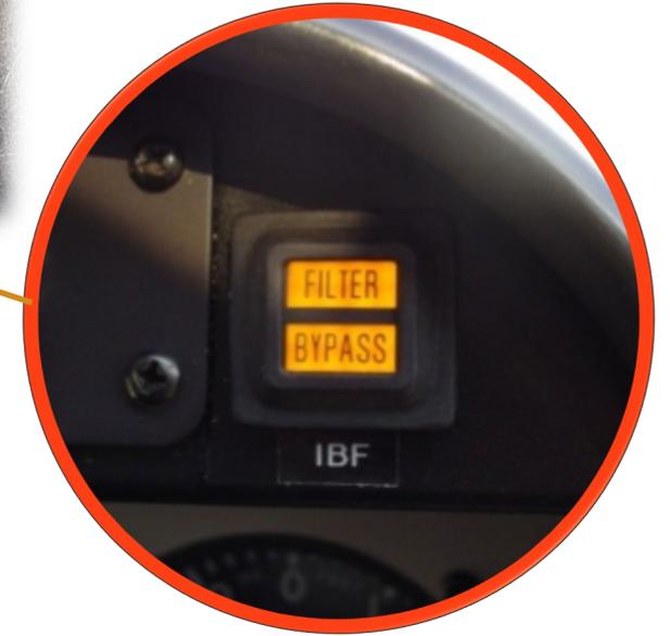
Pilot commands the bypass door to open to increase engine airflow until clear of debris conditions.
