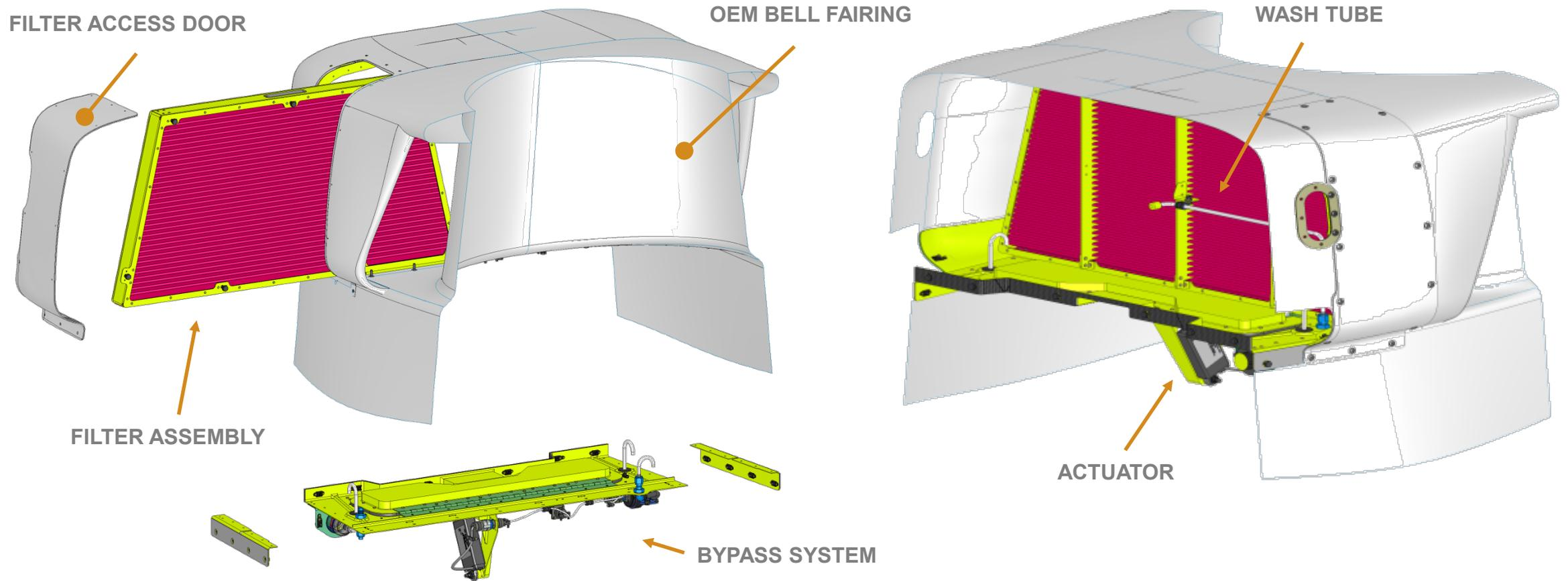
SHOWN INSTALLED INTO BELL FAIRING, LOOKING AFT. IBF UTILIZES EAPS MOUNTING PROVISION.
