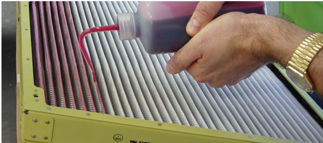
Picture 4: Oiling Filter Media
