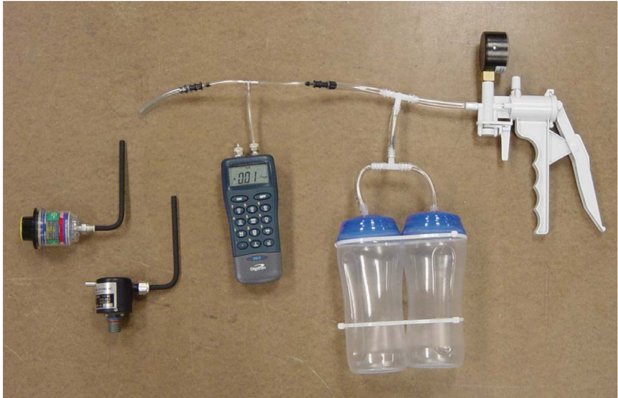
Picture 6: Test Setup with Manometer
