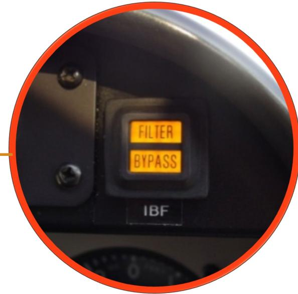
Pilot commands the bypass door to open to increase engine airflow until clear of debris conditions.
