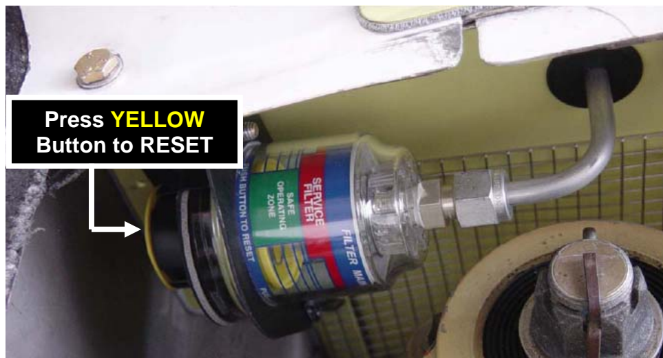
Figure 2-1. FILTER MAINTENANCE AID – (ABOVE) “YELLOW Indicator” position relative to SAFE OPERATING ZONE (“GREEN Zone”) or SERVICE FILTER (“RED Zone”) markings defines current filter condition and pushing “YELLOW RESET Button” resets indicator. (BELOW) FMA unit is mounted to front of the upper plenum of IBF assembly and is accessed through access hole in the cover plate.
