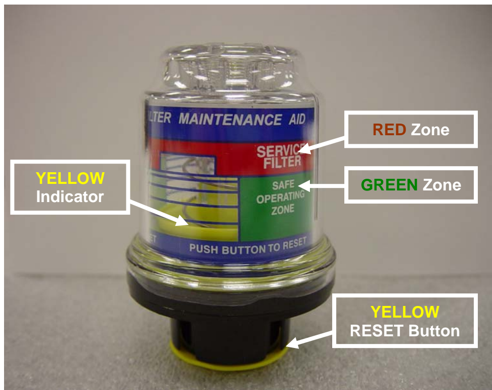
Figure 2-1. FILTER MAINTENANCE AID – (ABOVE) “YELLOW Indicator” position relative to SAFE OPERATING ZONE (“GREEN Zone”) or SERVICE FILTER (“RED Zone”) markings defines current filter condition and pushing “YELLOW RESET Button” resets indicator. (BELOW) FMA unit is mounted to front of the upper plenum of IBF assembly and is accessed through access hole in the cover plate.
