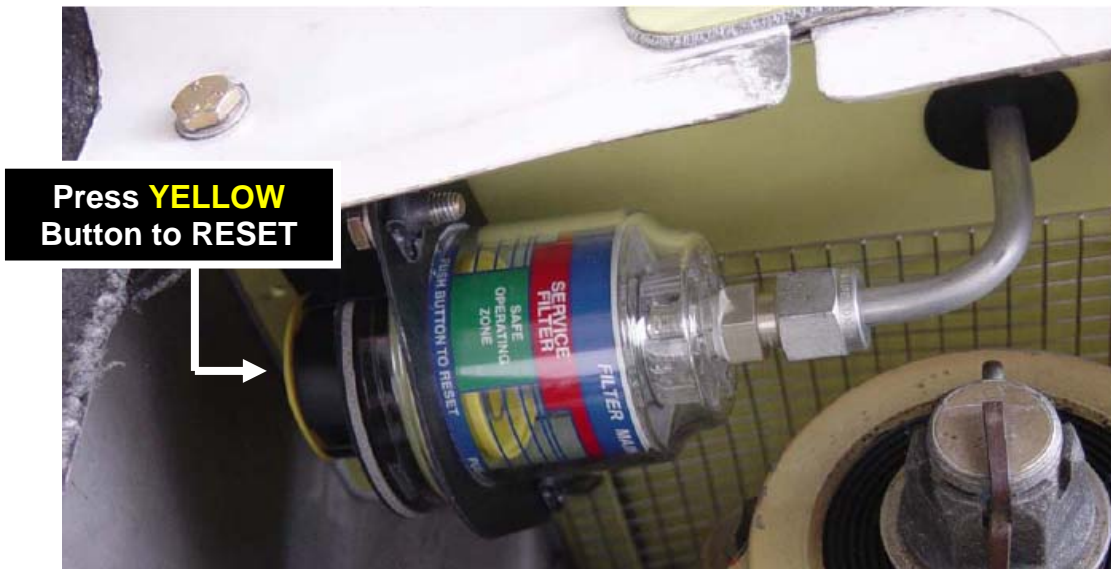
Figure 2-1. FILTER MAINTENANCE AID – (ABOVE) “YELLOW Indicator” position relative to SAFE OPERATING ZONE (“GREEN Zone”) or SERVICE FILTER (“RED Zone”) markings defines current filter condition and pushing “YELLOW RESET Button” resets indicator. (BELOW) FMA unit is mounted to front of the upper plenum of IBF assembly and is accessed through access hole in the cover plate.
