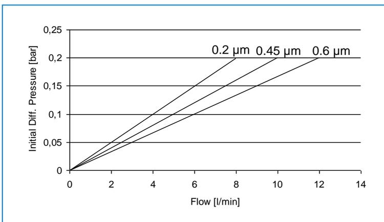
Data given for type UFTD-S PF-PES “W” with 3/8” connection.
