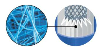
Cross section of the depth filter with SEM micrograph of the filter media
