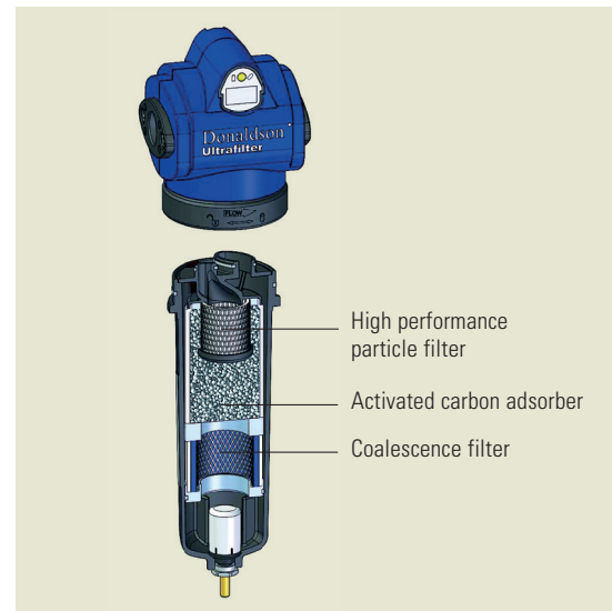
Cross-section of an DF Filter with DF-T element
