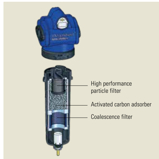
Cross-section of an Ultra-Filter with DF-T element
