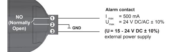
Alarm output for remote control, max. current 0.5 A.
