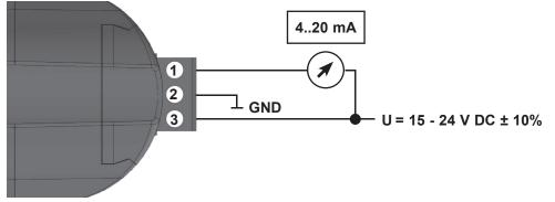
Output for data transmission. Analog output 4-20 mA, output resistance max. 500  $\Omega$ .
