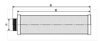
\* Uf-plug connection with double-o-ring
