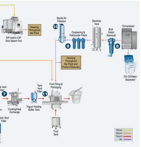
temperature changes during sanitation or sterilization. In order to ensure that the makeup air is safe and sterile, use a P-BE tank vent housing with P-SRF V element.
