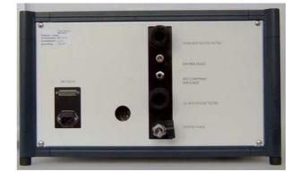
The aerosol generator provides a constant supply of test aerosol. The test aerosol is checked by the system when the FTC is started and in fixed intervals.
