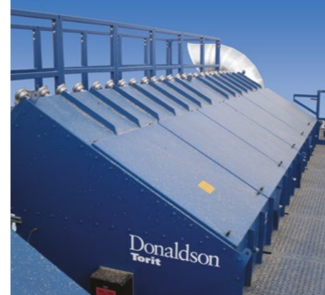
CPC - Grain Tipper Conveyor 31,765 m 3 /h (18,700 cfm)
