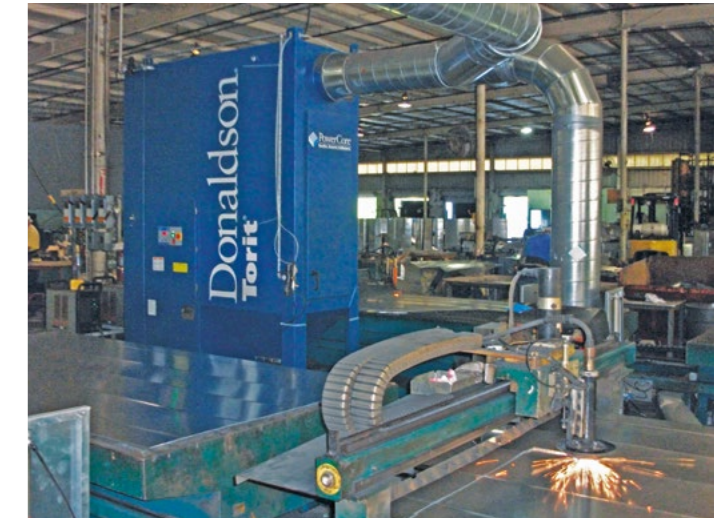
TG on Plasma Cutting 5,775 m 3 /h (3,400 cfm)
