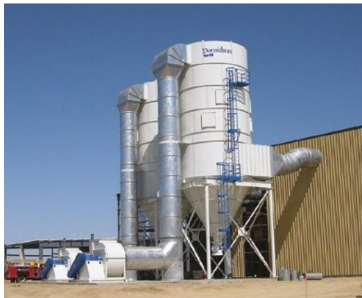
LP on Nut Dust 475,622 m 3 /h (280,000 cfm)
