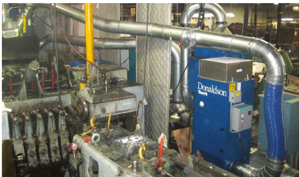
WSO on Cold Forming 2,038 m³/h (1,200 cfm)
