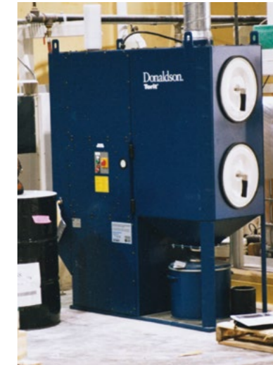
DFO on Paint & Pigment 2,038 m³/h (1,200 cfm)
