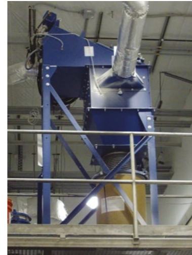
CPC on Milk Powder 2,038 m³/h (1,200 cfm)
