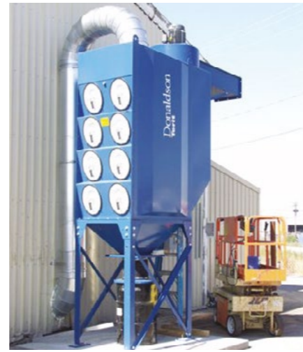
DFO on Plasma Cutting 8,493 m 3 /h (5,000 cfm)
