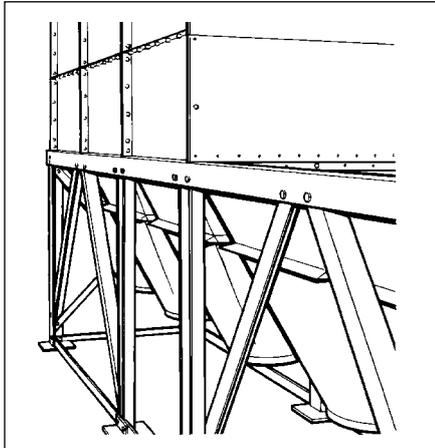
Figure 12 Place filter case on hopper/support flanges
