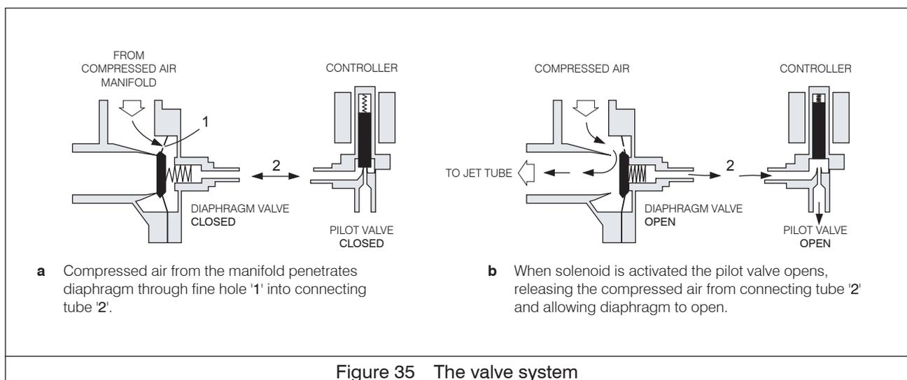
Figure 35 The valve system
