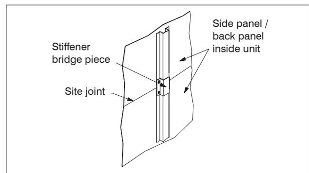
Figure 20 Part view showing typical position of stiffener bridge piece
