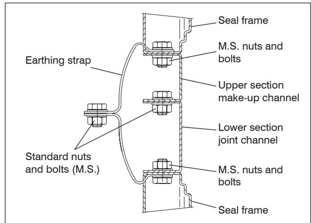
Figure 28 Typical upper and lower section joint showing earthing arrangement
