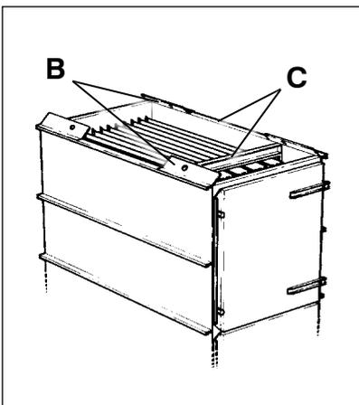
Figure 14 Remove lifting brackets on lower sections
