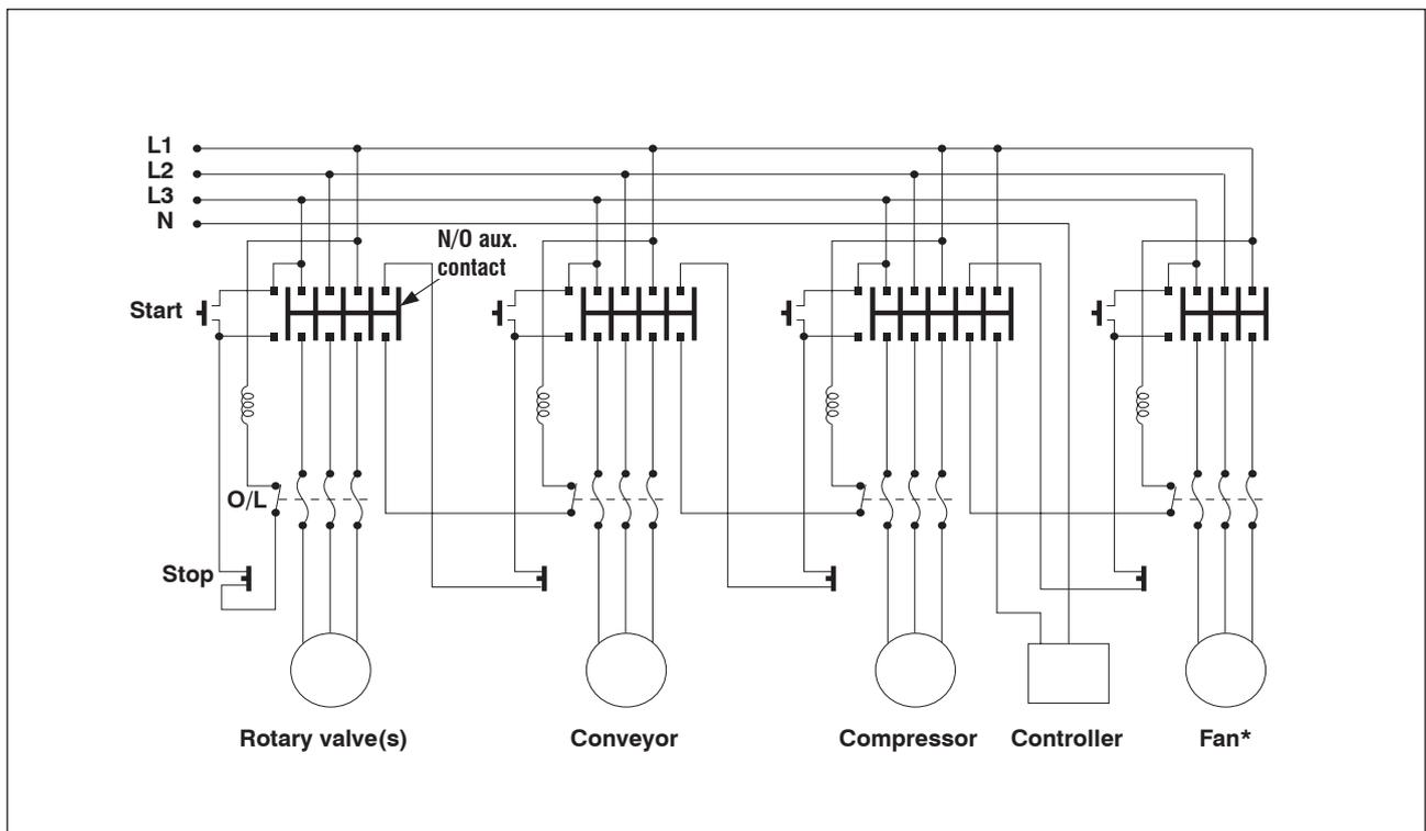
Figure 26 Schematic diagram showing typical interlock system for a Dalamatic collector installation
