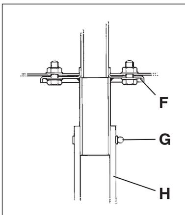
Figure 22 Hose stem adaptor fixing
