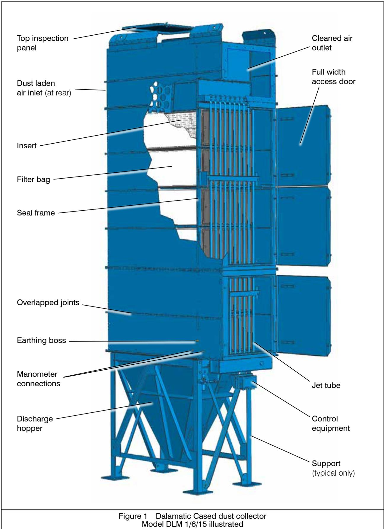
Figure 1 Dalmatic Cased dust collector Model DLM 1/6/15 illustrated
