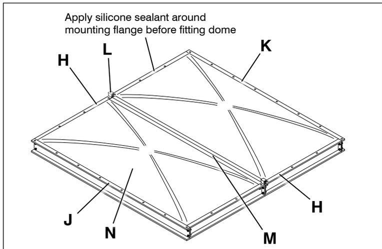
Figure 18 Erect explosion dome (2-bank shown)
