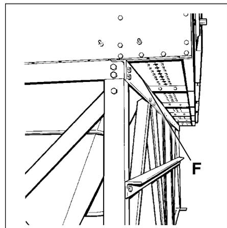
Figure 16 Clean air chamber base / hopper joint
