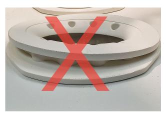
12. If the filter is not seated completely against the tubesheet (see below), the insert will need to be taken out and the filter pressed down. Once the filter is properly seated, the insert can be reinstalled.
