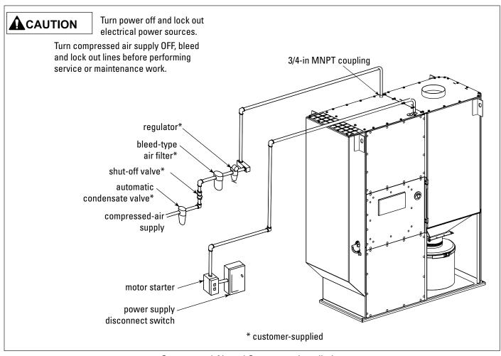
Compressed Air and Component Installation
