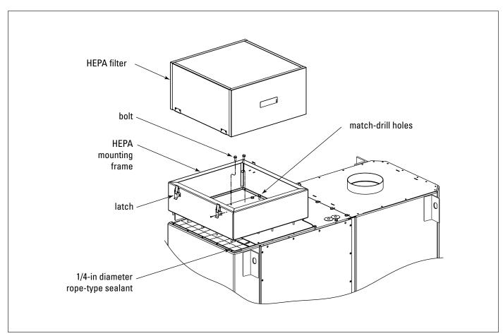
**HEPA Afterfilter Installation**
