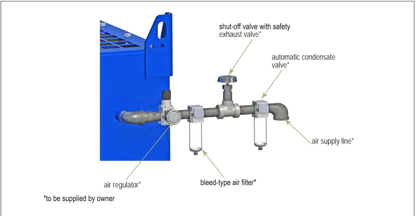
Compressed Air and Component Installation
