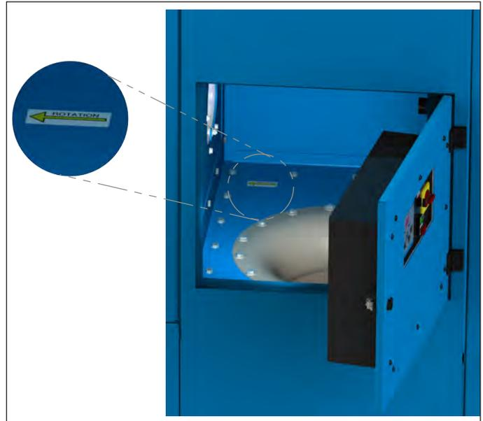
3. If the fan rotation is reversed, correct the rotation.
