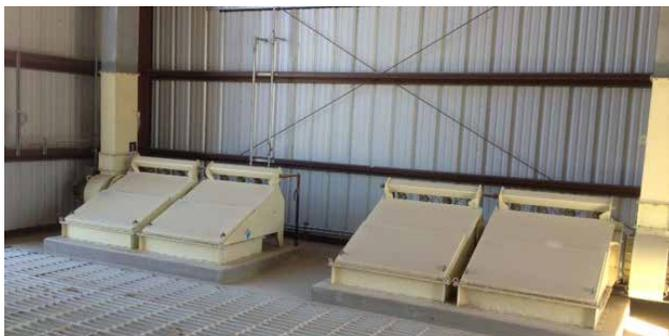
For new or replacement dump pits, **3** PowerCore CPV collectors require smaller, quieter fans that reduce noise exposure and lower costs.
