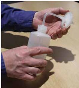
2. Install solvent\* dispensing tube and install solvent filter on end of the dispensing tube.
