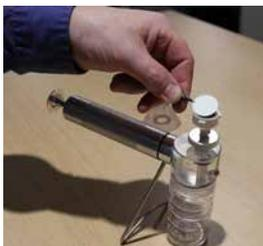
4. Separate the funnel from the patch supporter and install a filter patch with ink grid up. (If the patch has an ink grid).
