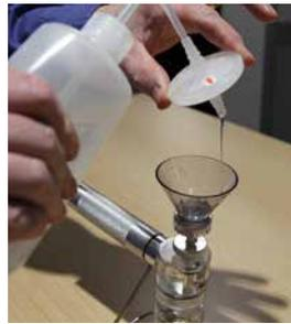
8. Once the entire sample has passed through the patch rinse the funnel with filtered solvent and draw through the patch. Continue to pull air through until the patch starts to dry. Then separate the funnel from the patch supporter and remove the patch with forceps.
