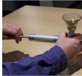
7. Draw the sample fluid through the patch by pulling on the vacuum pump handle.
