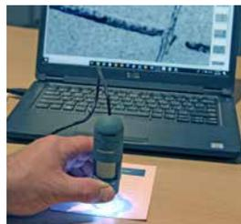
10. Analyze the sample with the 100x magnification field microscope.
