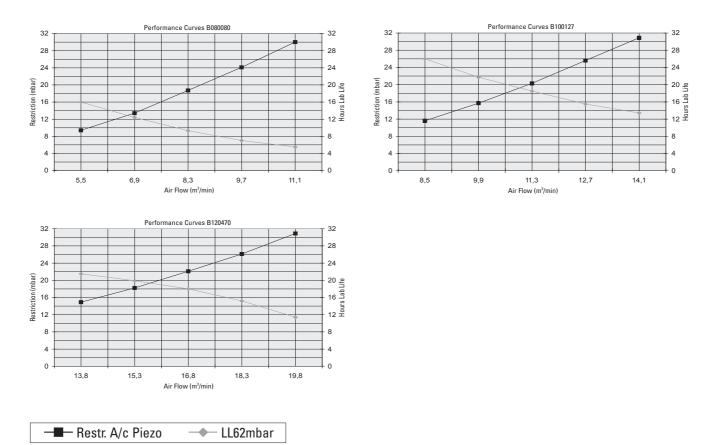
All performance curves are according ISO 5011 standards - Restriction measured at Piezo All tests are done with ISO Coarse at Dust Concentration of 1g/m<sup>3</sup>
