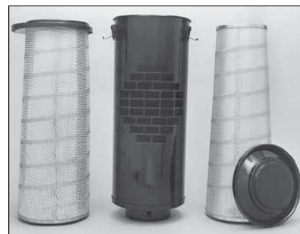
ECG Konepac with Perforated Inlet — an alternative to disposable style housings. You'll get the economy of replacing the filter instead of the entire unit each time. The perforated inlet on the side of this G112417 housing (middle) is the same as the disposable's, so conversion is direct and easy. Left: Extended service filter. Right: Filter designed for scheduled maintenance.
