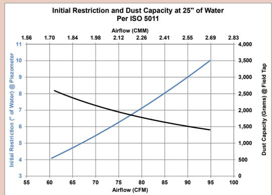
\*Results generated using laboratory testing pursuant to ISO5011. Actual performance during use may vary depending on multiple factors, including specific product configuration, external conditions and application.
