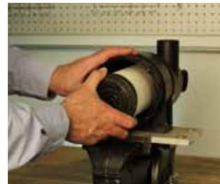
*If you perform filter maintenance service on a schedule versus using service indicators, you may want to write the service date on the end cap of both filters.*
