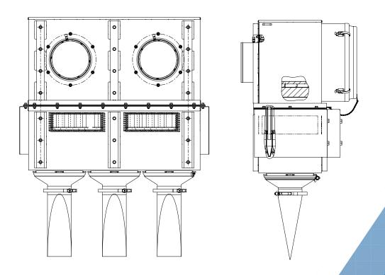
The SSG air cleaner series is a family of two-stage RadialSeal™ engine air cleaners that provide improved reliability and better durability compared to axial seal style air cleaner designs.
