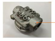
Donaldson filter head assembly P506139 has  $3 \times 1/8$ " BSP gauge ports. The gauge should be installed into the upstream ports on the top of the head. We recommend the use of fuel resistant thread sealant on the gauge thread.
