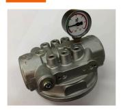
Screw the gauge firmly into the gauge port. Gently tighten with a correctly sized spanner until the gauge is correctly oriented for viewing. Do not over-tighten.
