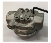
Using a correctly sized tool, undo the port plug in the top port by rotating in an anti-clockwise direction
