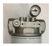
The gauge is only intended for use with a pump. When the filter is new, the gauge will display the fluid pressure before the filter. As the P579099 filter loads with contamination, this pressure will gradually increase. The filter should be replaced when the flow pressure exceeds 25psi, or reaches the maximum pressure of the delivery pump, whichever is lower, or when the flow rate becomes unacceptably slow.
