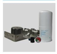
The filter in this kit is manufactured with water absorbing media designed to filter particles 10um (micron) @ b200, providing you with added protection against particulate and water contamination in your fuel.
