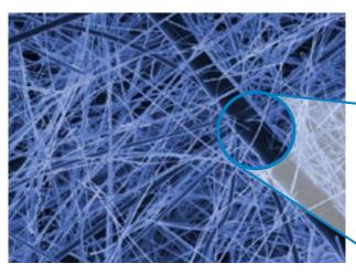
Donaldson's proprietary Synteq  $XP^{m}$  nanofiber media creates small, consistent inter-fiber spacing – increasing filter capacity.
