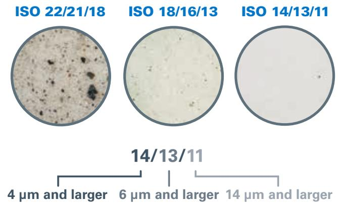
A finer micron filter will collect smaller contamination from the fuel and may reach its dirt holding capacity more quickly. It may need replacing more often than a larger micron filter.
