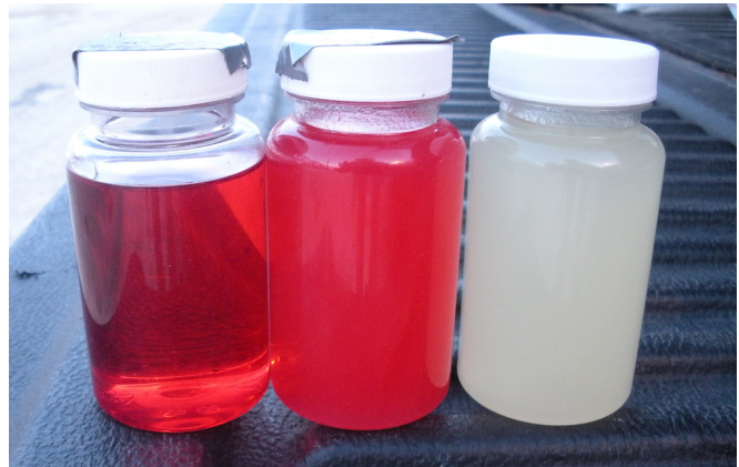
Upper Midwest (United States) diesel fuels stored at -23^{\circ}\text{C} / -9^{\circ}\text{F} (left to right). #1 off-road, #2 off-road, and #2 on-road. Both #2 samples have been treated with cold flow additive and still show significant filterable paraffin-wax solid formation. See Strategy 1.
