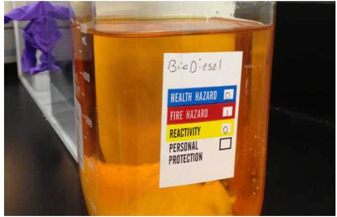
Midwest (United States) produced Soy B100 stored at 4°C / 40°F. The solids in the bottom are glycerin fallout and would plug most any filter. See Strategy 9.
