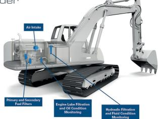
Donaldson is expanding its Filter Minder wireless monitoring system, which began with engine air filters, to incorporate literally all the types of air and liquid filtration technologies found on vehicles and equipment.
