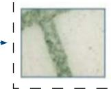
ISO 16/14/11 Target rating for hydraulic/ transmission oils
