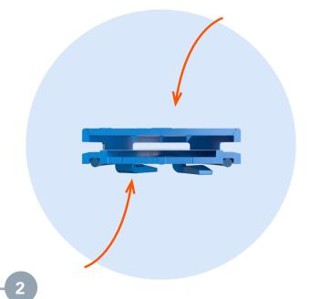
In the case of rapid pressure and heat buildup, the second stage helps maintain internal enclosure pressures by allowing gases to escape by either bypassing the membrane with the umbrella flex or bursting the membrane.
